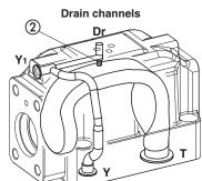
Internal piloting: Without blinded plug SP-X500F ①; External piloting: Add blinded plug SP-X500F ①; Without blinded plug SP-X300F 2; Internal drain: External drain: Add blinded plug SP-X300F 2.
