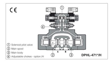
Spool type, pilot operated directional solenoid valves available in 4/3, 4/2, 3/2 way versions.
