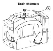
Internal piloting: Without blinded plug SP-X300F ①; External piloting: Add blinded plug SP-X300F ①; Without blinded plug SP-X300F @; Internal drain: Add blinded plug SP-X300F 2. External drain:
