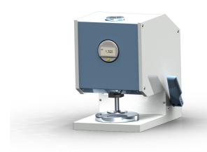
It is manufactured by us from a sturdy and robust case. The DM 2000 is your choice if you value accurate resolution (up to 0.001 mm), high measuring accuracy, good handling and permanently reproducible and objective results.
